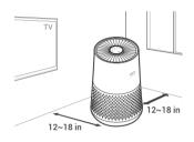
Allow 12 ~ 18 in. of space between TVs, radios, and other electronics Electromagnetic interference from certain electronics may cause product malfunction
