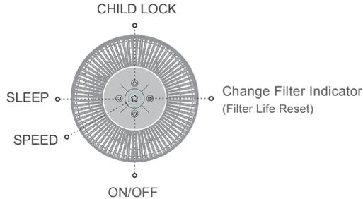
**On power on state, the device enters in standby mode when ON/OFF indicator light turns red**
