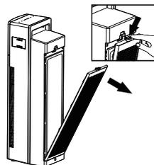
Step 3: Remove the used combination filter and wrap it with polybag to avoid the pollutants spread indoor.
