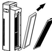
Step 4: Insert new combination filter into the unit. Consult the arrow on the filter for correct installation direction.
